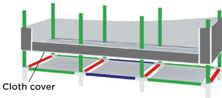
2. Put the cloth cover along the long tube, noting that the bottom layer of the cloth cover is separated by white layer cloth on top.
