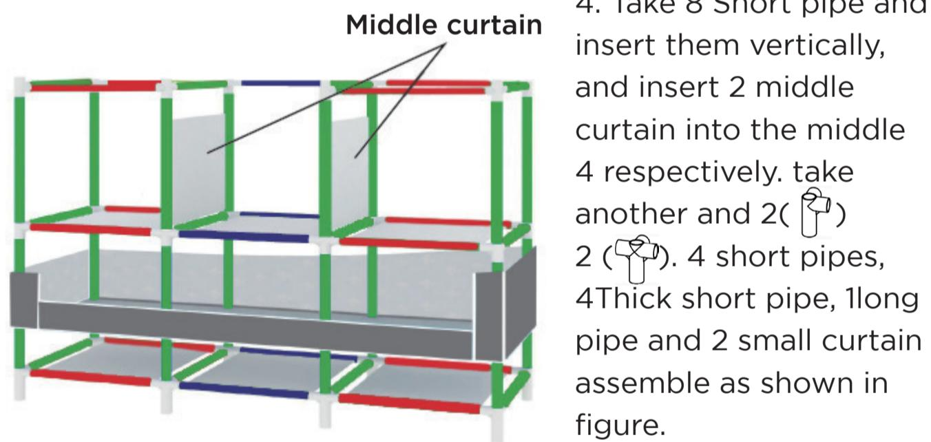
4. Take 8 Short pipe and insert them vertically, and insert 2 middle curtain into the middle 4 respectively. take another and 2( ). 2 ( ). 4 short pipes, 4 Thick short pipe, 1long pipe and 2 small curtain assemble as shown in figure.
