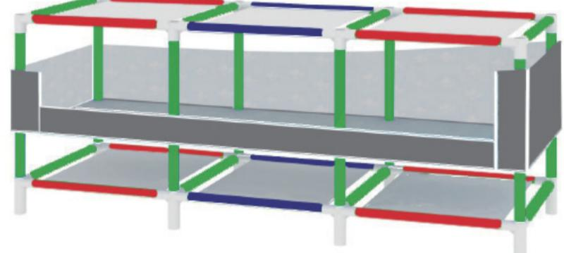
3. Take 4 ( ), 4 Thick short pipe, 4 Short pipe, 2 long pipe, 2 small curtain and 1 big curtain assemble as shown in figure.
