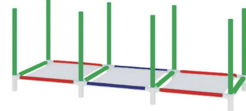
1.Take 4 ( ), 4 Thick short pipe, 4 Short pipe, 2 long pipe, 2 small curtain and 1 big curtain after installing the bottom layer, take 8 short pipes and insert them vertically ( ) and ( ) top.
