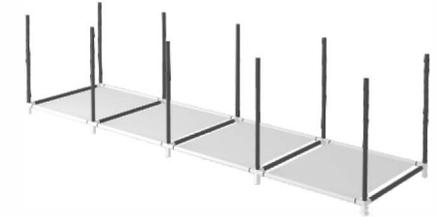
2. Insert 10 steel pipes.
