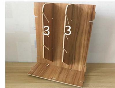
Take the wood n°2 and n°3 and insert them in n°2 as shown in the picture and fix it by means of the screws.
