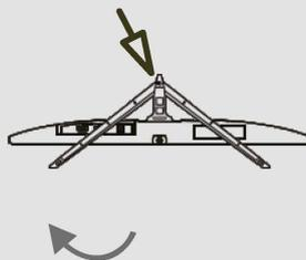
Unscrew the screws at the bottom of the bracket to remove it.
