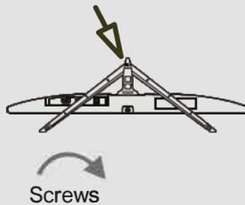
Place the screws at the bottom of the base and tighten them with a screwdriver.
