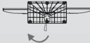
Unscrew the screws located at the bottom of the bracket to remove it.
