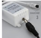
Plug the DC12V power supply into the controller
