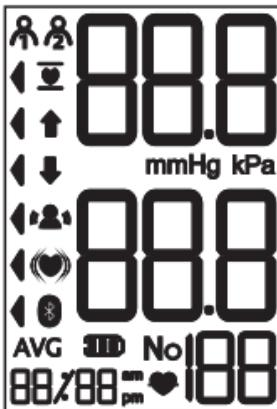
Note: Unit will not function if residual air from previous testing is present in cuff. The LCD will flash "↓" until pressure is stabilized.
