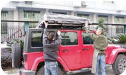
3) Adjust the tent to the appropriate position on the car roof. (Remember to make sure the trunk door can be opened)
