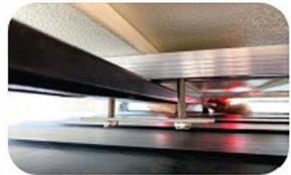
4) Slide the all bolts with slip fixed to appropriate position on the connecting tube. Please be noted, when the distance between roof rack and car roof is less than 4cm, the short bolts will be used instead of the long bolts.
