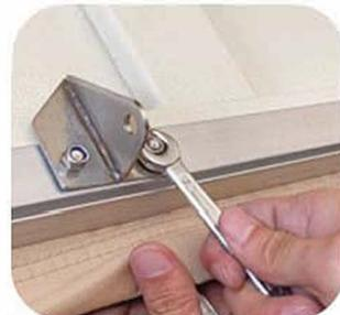
2. The long screw passes through the screw hole under the bed plate and fasten the nuts tightly.
