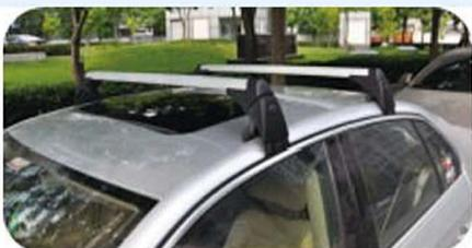
C.Fixing the transverse roof racks on the door frame.
