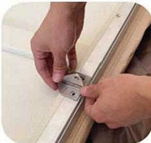
1. Align the ladder connector with screw holes on the bed plate.
