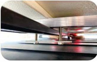
5) Put the black plastic in the middle of rack and U-shaped fixing and make the bolts with slip fixed on the U-shaped fixing plate, then tighten the plastic self-locking nut by hands. Please be noted total 4 pcs U-shaped fixing plates should be fixed on 4 sides respectively
