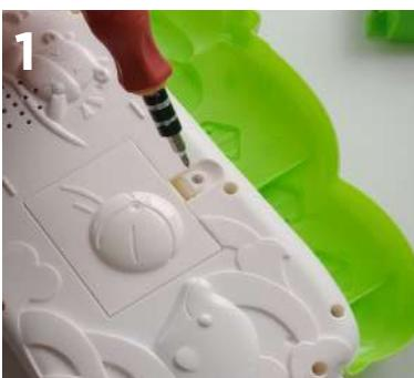
1 - The battery compartment is located at the rear of the piano. Using a screwdriver, remove the screw and remove the cover.
