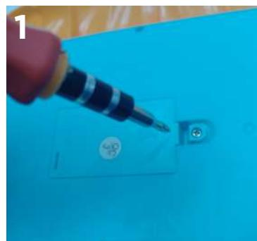
1 - The battery compartment is located at the rear of the piano. Using a screwdriver, remove the screw and remove the cover.
