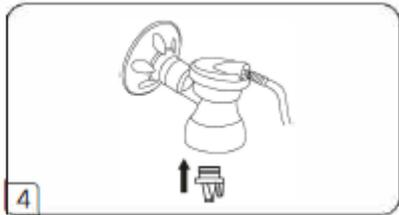
Put the duckbill valve into the bottom outlet of the three-way to ensure that there is no leakage.
