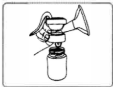
5. Put the bottle in the bottle mouth screw threaded through the bottom of the pump connector
