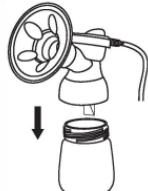
5. Screw the three-ways assembly onto the bottle.
